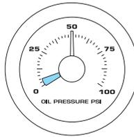
Do not continue to operate your engine as long as the pointer is in the red section. Otherwise, your engine may be severely damaged.
