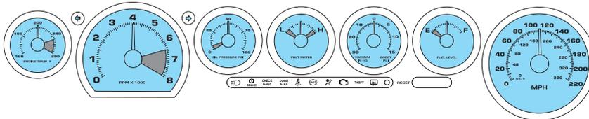
**Engine coolant temperature gauge:** Indicates engine coolant temperature. At normal operating temperature, the needle will be outside the red section. **If it enters the red section, the engine is overheating. Stop the vehicle as soon as safely possible, switch off the engine and let the engine cool.**
