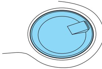
4. Insert fuel nozzle fully into the filler pipe using the nozzle to slide the plastic cover to the side.
