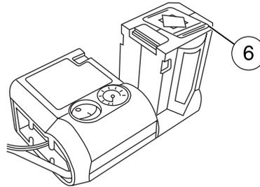
7. Turn the air compressor on by pressing the "I" side of the orange button.
