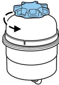
5. If the fluid is low, add fluid in small amounts, continuously checking the level until it reaches the range between the MIN and MAX lines. Be sure to put the cap back on the reservoir.
