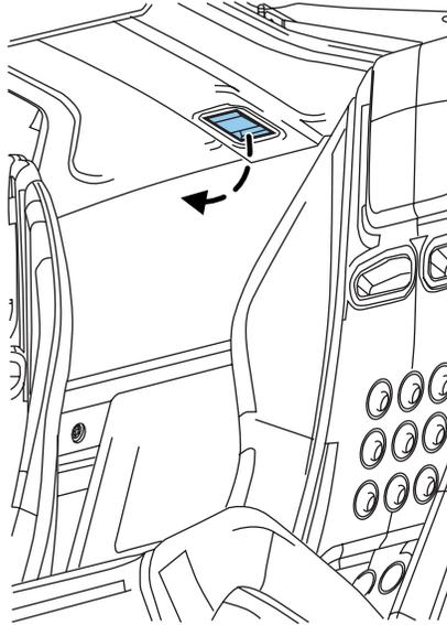
2. Lift up on the decklid at the side air scoop area to provide better access to the auxiliary release.
