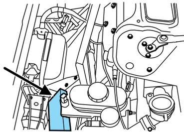
**Note:** The luggage compartment liner must be removed to access the power distribution box. Refer to *Removing the luggage compartment liner* in the *Maintenance and Specifications* chapter.
