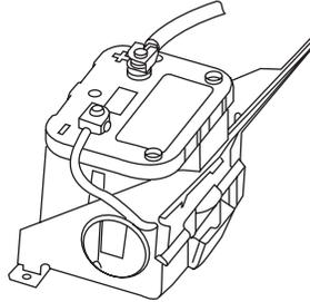
For longer, trouble-free operation, keep the top of the battery clean and dry. Also, make certain the battery cables are always tightly fastened to the battery terminals.
