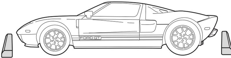
**Note:** Because of low vehicle ground clearance, use caution when approaching curbs/curb stops from front and rear — vehicle damage could occur.
