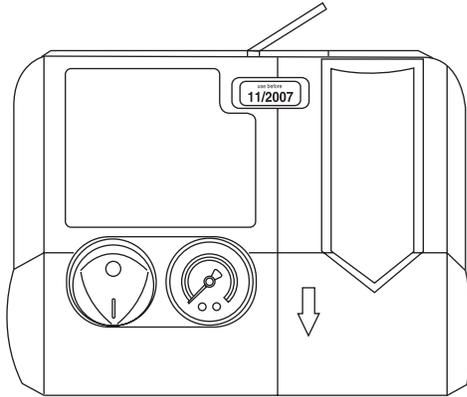
Your vehicle is equipped with an emergency tire inflation kit (located in the luggage compartment). The inflation kit consists of an air compressor to reinflate the tire and a sealing compound that will effectively seal most punctures caused by nails or similar objects. This kit will provide a temporary seal allowing you to drive your vehicle up to 120 miles at a maximum speed of 50 mph.
