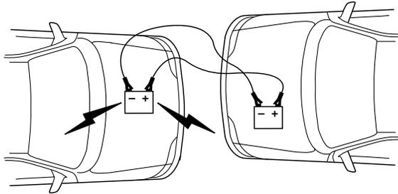
4. Make the final connection of the negative (-) cable to the negative (-) battery terminal of the stalled vehicle.
