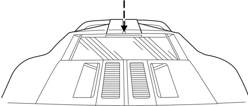
1. Pull the decklid downward to the secondary latch position. Push down on the center of the decklid firmly to close.
