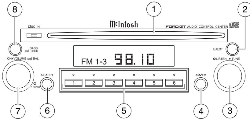
**A flashing anti-theft indicator (Disc in lamp), may be activated and de-activated by pressing and holding the CD Eject control for two seconds or more with the radio turned off.**
