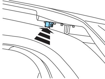
4. Go to the other side of the vehicle and release the right side auxiliary latch located behind the passenger seat area. Note: make sure not to relatch the driver's side.
