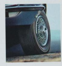
Tires. Included are Fiberglass Belted F70-14's with extra-narrow whitewalls; black sidewall E78-14's, and white sidewall C78 or E78-14's. Also available: widetread radial ply FR70-14's with narrow white sidewalls.
