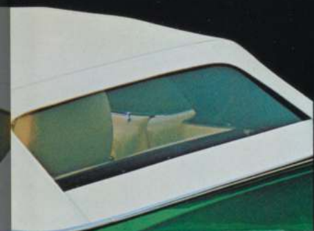
CONVERTIBLE POWER-OPERATED TOP is of padded, 5-ply vinyl. Solid, tempered-for-strength glass backlite resists scratching, won't fade or discolor.
