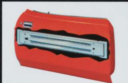
Steel Guard Rail —standard on all 1971 Mustangs. Steel box-section door beams help absorb side impact forces.
