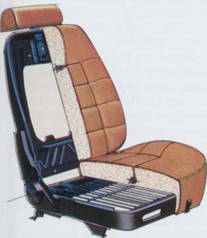
Mustang's front bucket seats combine foam padding over a spring steel base with the warmth of cloth and the individual comfort of reclining seat backs.
