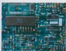
Ford's new EEC-IV computer provides precise and instantaneous control over vital engine functions.
