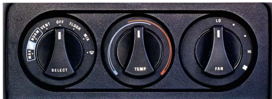
Air conditioning with rotary controls.
