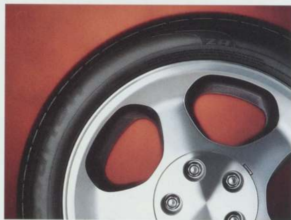
The Cobra's 17.0-inch five-spoke alloy wheels are wrapped with BFGoodrich Comp T/A ZR radials, which are derived from the Comp T/As fitted to SVT's 1995 Mustang Cobra R race car.
