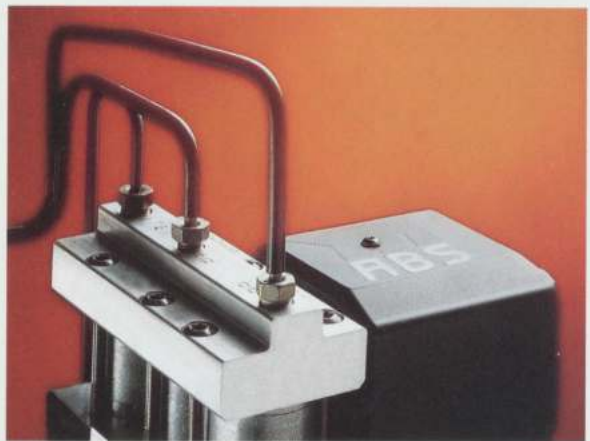
The Cobra's brakes are monitored and controlled by a three-channel, four-sensor Bosch ABS system that can modulate and adjust each of the four calipers every 10 milliseconds.
