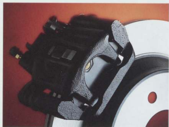
The 11.65-inch rear brakes are clamped by single-piston calipers. The rotors feature internal cooling vanes.
