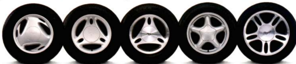
Left to right: 15" wheel cover (standard on Mustang); 15" cast aluminum wheel (optional on Mustang); bright machined 15" optional wheel; 16" cast aluminum wheel (standard on GT); 17" cast aluminum wheel (optional on GT).
