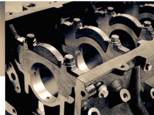
The 4.6-liter Mustang GT crankshaft features durable four-bolt main bearing caps.
