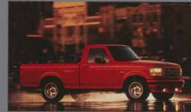
1993-1995 SVT F-150 LIGHTNING 240 horsepower 5.8-liter ohv V8 E4OD four-speed automatic transmission Tow rating: 5,000 lbs.; payload: 745 lbs. Production: 11,563 Units
