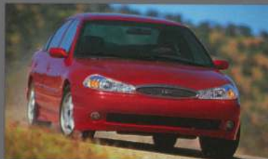
1998-1999 SVT CONTOUR 195 hp ('98), 200 hp ('99) High Output 2.5 liter Duratec V6 MTX-75 five-speed manual transmission Front-drive, five passenger sports sedan Production: 8,535 units (estimate)
