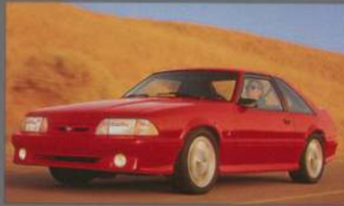
1993 SVT MUSTANG COBRA 235 horsepower 5.0-liter ohv V8 T5 five-speed manual transmission Four-wheel disc brakes Production: 4,993 units
