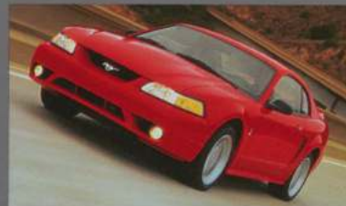
1999 SVT MUSTANG COBRA 320 horsepower 4.6-liter dohc V8 Independent rear suspension introduced Traction control introduced Production: 8,000 units (estimate)
