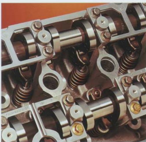
The SVT Cobra cylinder heads follow classic double-overhead cam design.
