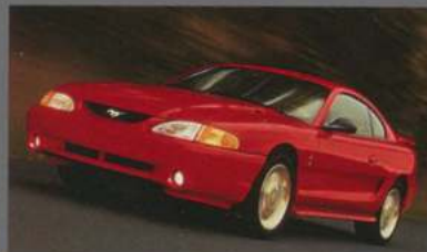
1994-1995 SVT MUSTANG COBRA 240 horsepower 5.0-liter ohv V8 T5 five-speed manual transmission 13-in. front discs, PBR calipers; 11.65-in. rears Production: 11,017 units
