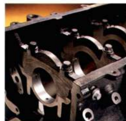
The 4.6-liter Mustang GT crankshaft utilizes durable four-bolt main bearing caps.
