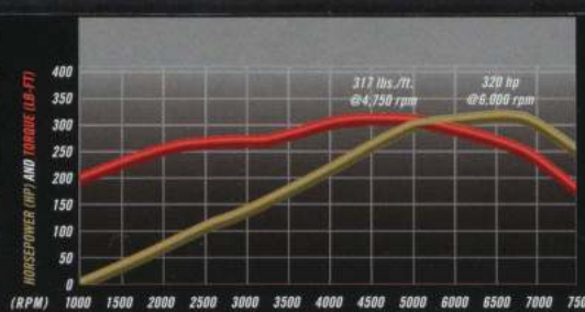
The SVT Cobra is free-revving from idle to its 6,800-rpm redline. It produces 320 horsepower at 6,000 rpm, and 317 lb.-ft. of torque at 4,750 rpm. The SVT Cobra V8 develops 69.55 horsepower per liter, or 1.14 horsepower per cubic inch.
