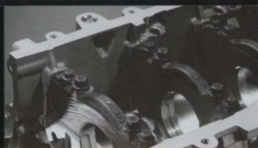
The main bearing caps that carry the forged crankshaft are secured to the lightweight aluminum-alloy block with six high-tensile steel bolts, spreading loads over a broad area of the block.
