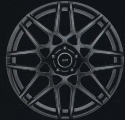
19" x 9.5" Front/20" x 9.5" Rear Tarnish-Painted Forged-Aluminum Included: Shelby GT500 SVT Performance Package
